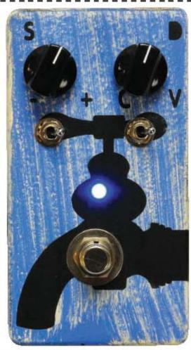
about 3/4 of the way up, resulting in what sounds like a minor second trill. By adjusting the speed, you can make the trill speed up and slow down. With the toggle switch set to the plus side, the individual notes in the trill interval get more defined. On the minus side, the notes get a little more slurred. It's a cool effect if you want to make single notes sound like trills up and down the fretboard.
